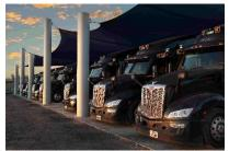
connects the two cities. This custom-built terminal will house, maintain, prepare, inspect, and deploy autonomous trucks. It is equipped to handle requirements specific to driverless operations such as sensor calibration ranges, high-speed data offload, and launching and landing zones. In common with the traditional trucking terminals, this terminal also has fueling and weigh stations as well as on-site maintenance facilities. More information is at this link.
