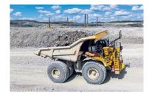
more. The trucks operate in special zones and use AI, GPS and sensors to navigate complex terrain, plot efficient paths, and avoid obstacles. Connected by Wi-Fi and cellular towers, autonomous trucks are supervised from an onsite control room. More information is at this link or this one.
